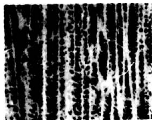
Figure 5-9: Iron-25% nickel alloy. Photomicrographs at 1", 2" and 4" from the chill. Casting 4, 34X.
