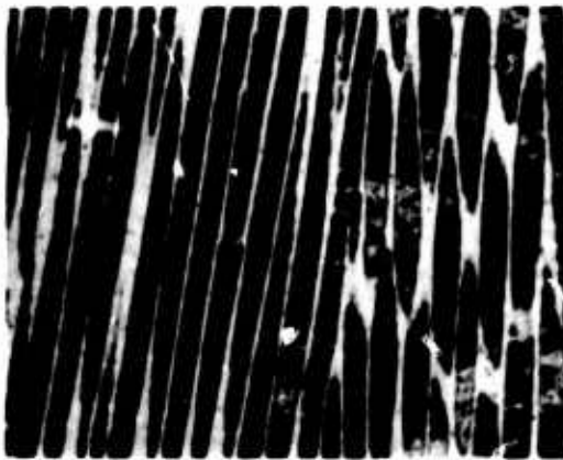
Figure 5-3: Iron-10% nickel alloy. Photomicrographs at 1", 2" and 4" from the chill. Casting 1, 34X.
