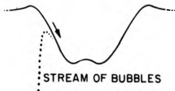
(E) OBSERVED REVERSE FLOW DOWN SIDE OF CRATER LEFT BY SOLID SPHERE
