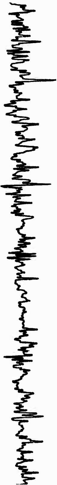
Figure 10. Noise recorded on 13 July 1965 on ocean bottom at 72° 03' W, 36° 11' N. Depth of water 3600m. Magnification 125K at 1 Hz
