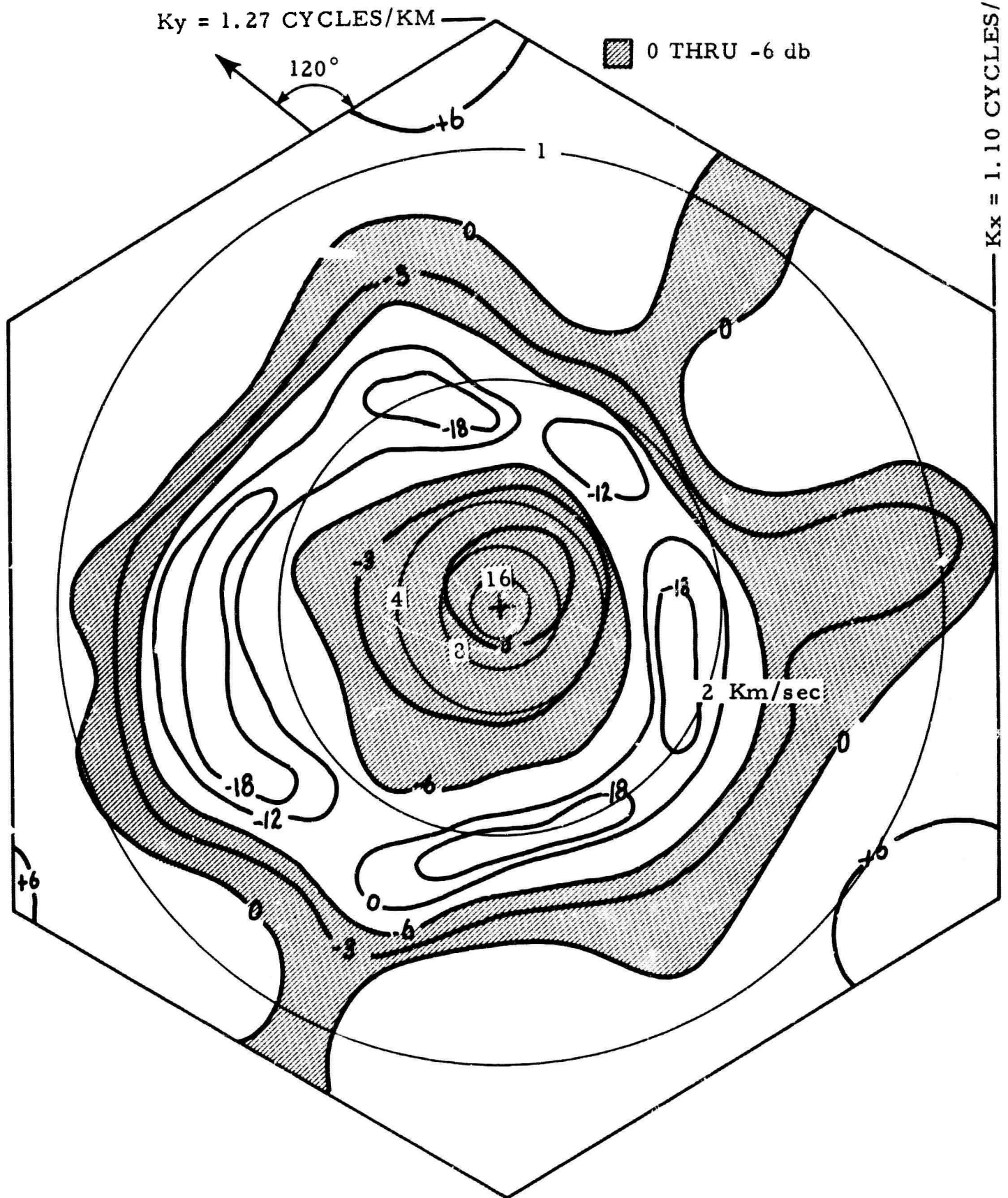
Figure VI-13. Two-Dimensional Wavenumber Response of UBO MCF-8, f = 1.0 \text{ CPS}
