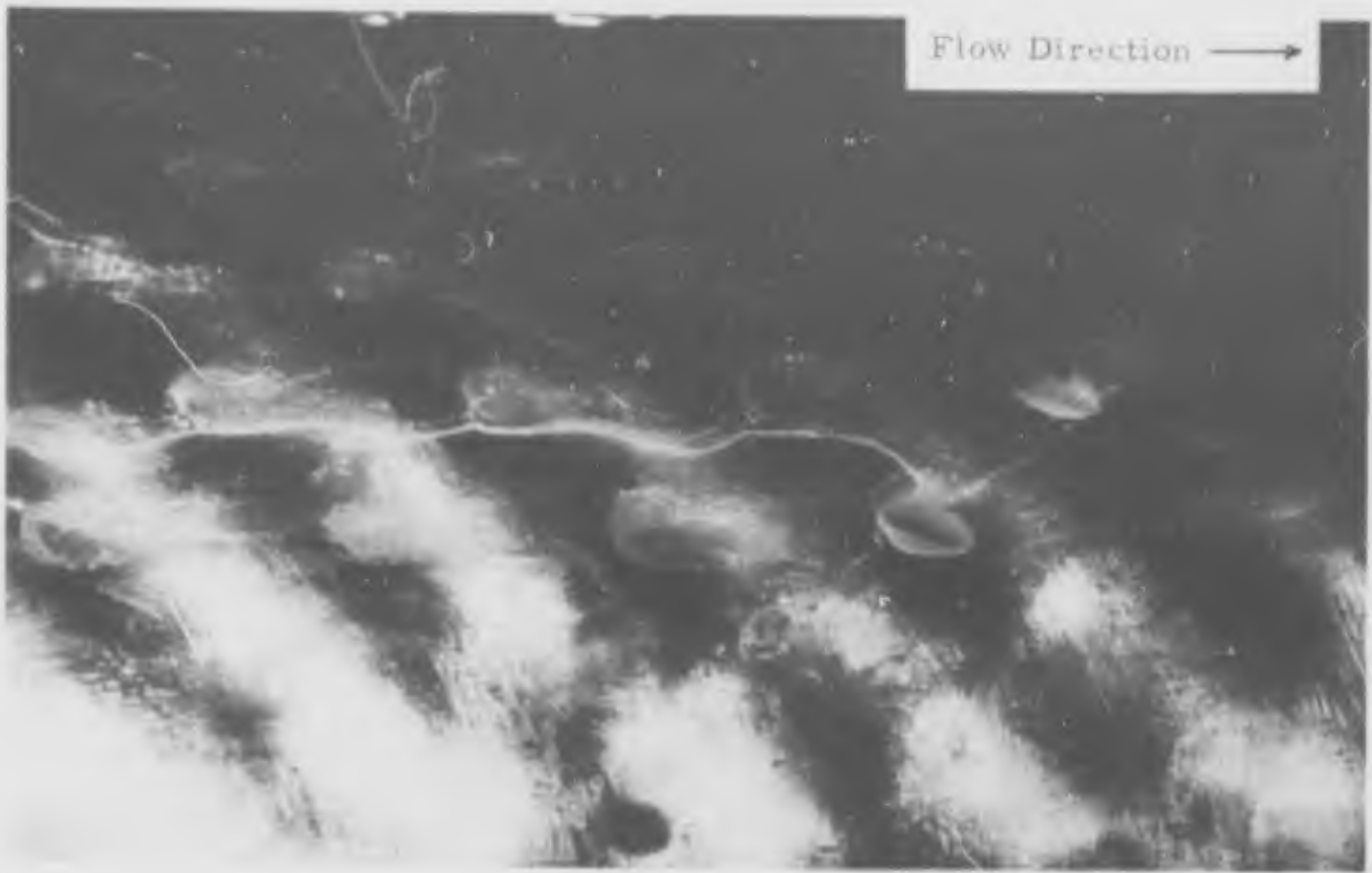
Fig. 16 Separated Flow on Model #20. ( M = 4.62 , P_t = 4000 psf.)
