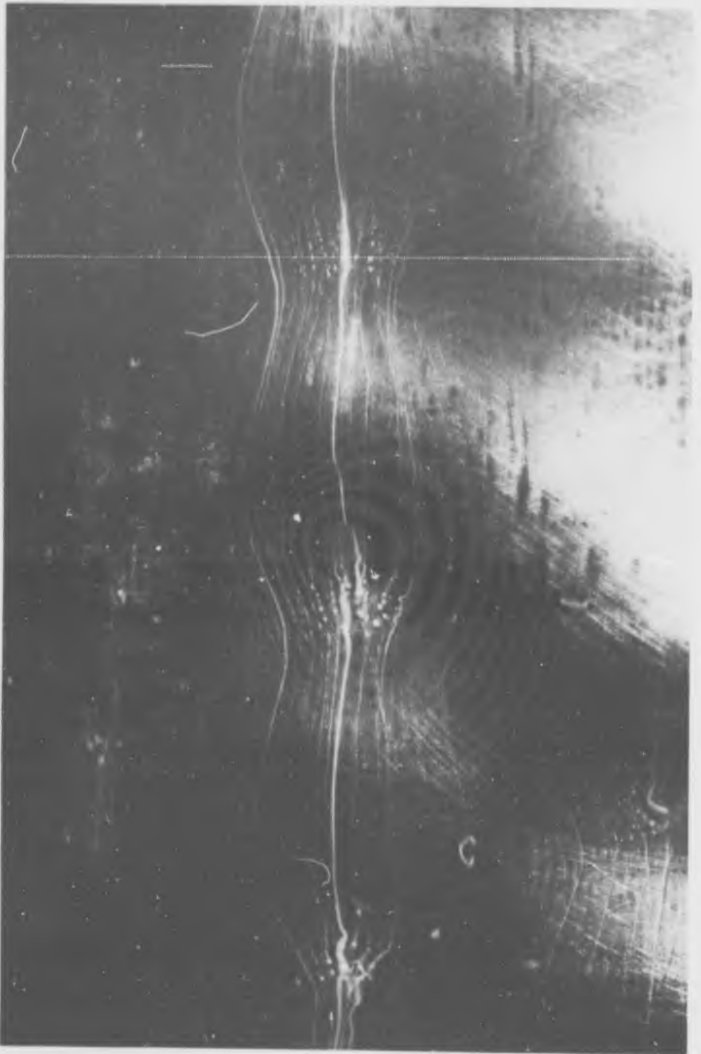
Fig. 11 Oil Film Study. Model #10 at Mach 3.0
