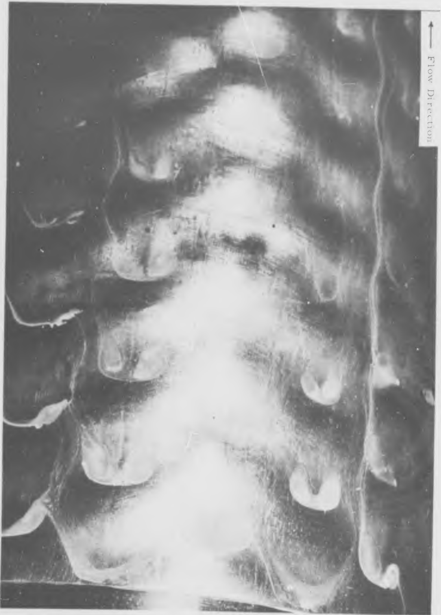
Fig. 15 Separated Flow on Model #10. ( M = 4.62 , P_t = 4000 psf.)
