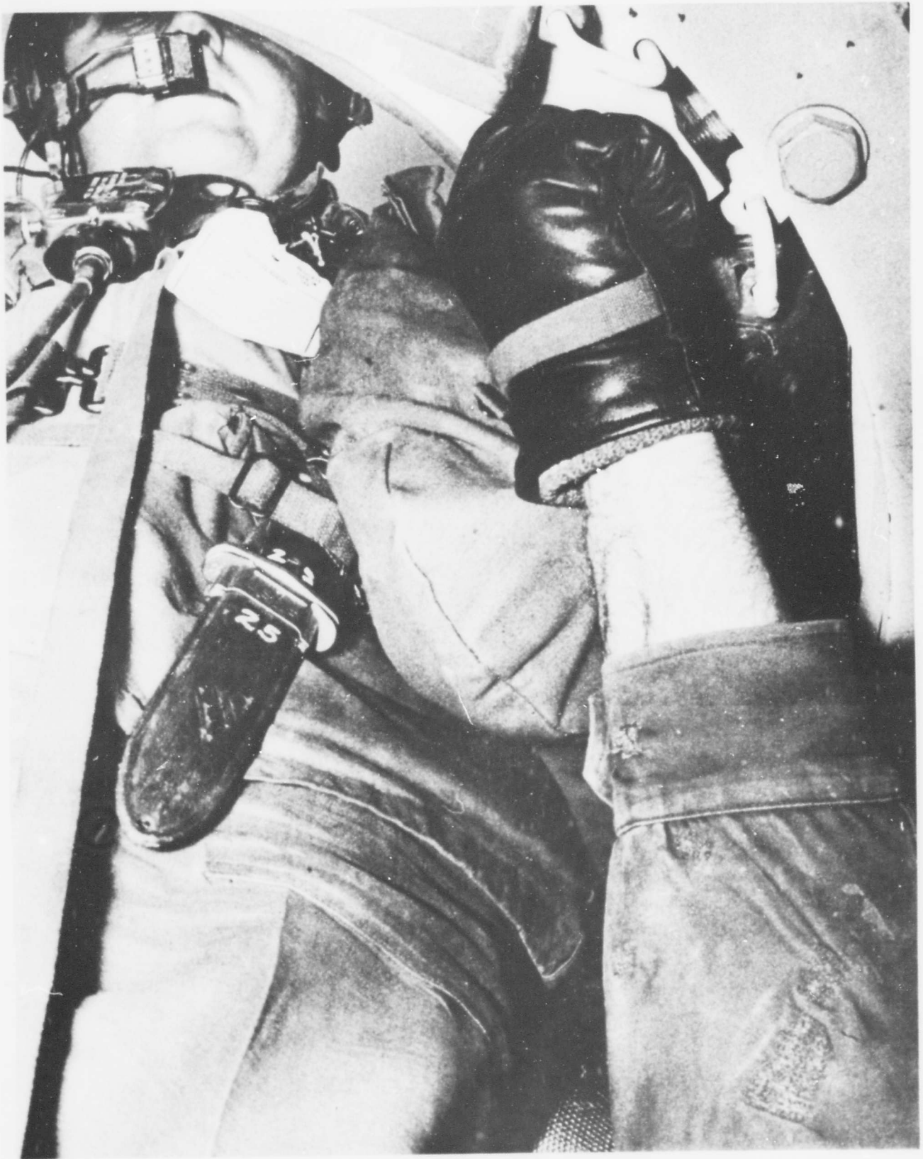
FIG 7. While riding over rough terrain, the Commander tried to tighten the cupola. After some delay he located the cupola lock. Due to his unfamiliarity with the mechanics of the cupola lock, he unscrewed the lock. This picture shows a squad member finally coming to his aid.
