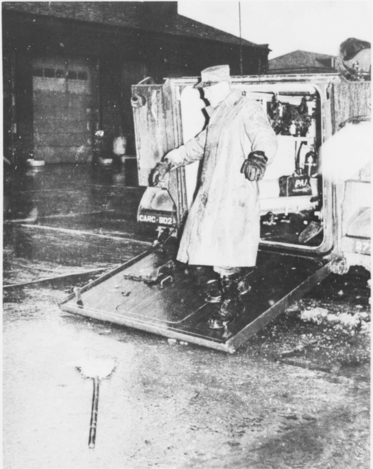
FIG 12. Soldier skidding on a wet ramp without any non-skid coating or horizontal bars.
