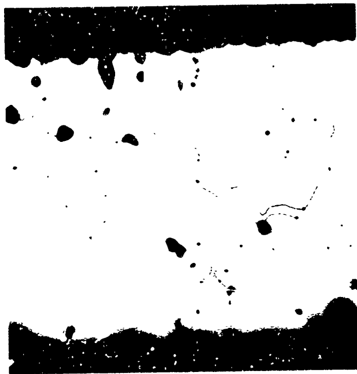
Fig. 2 99.99% Nickel strip heated 48 hours at 850°C in Na 2 SO 4 , evacuated capsule. 150X
