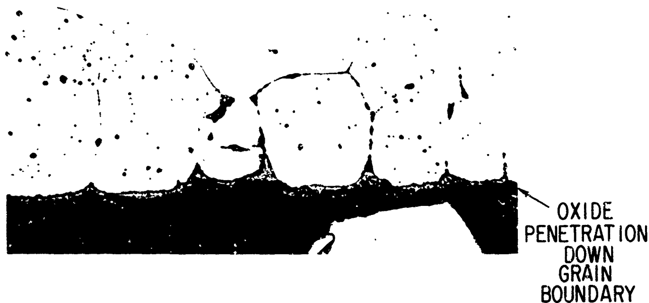
Fig. 11 "A" nickel sulfidized 4 hours at 250°C, then oxidized 4 hours at 850°C in air. 500X
