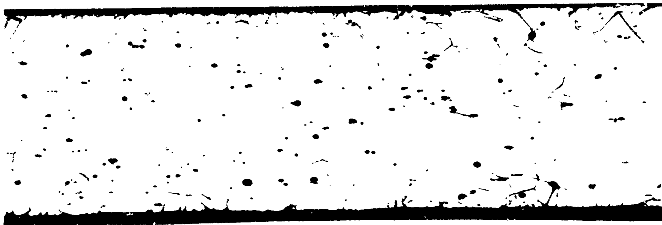
Fig. 9 Sodium sulfate-coated nickel exposed to argon at 805°C for 60 minutes (N221). 100X
