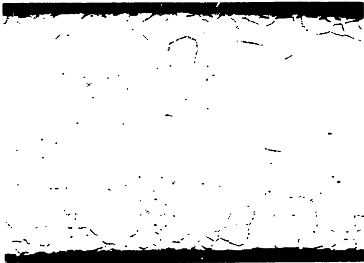
Fig. 6 "A" nickel heated 4 hours at 850^\circ\text{C} in \text{H}_2\text{S}/\text{H}_2 mixture.
