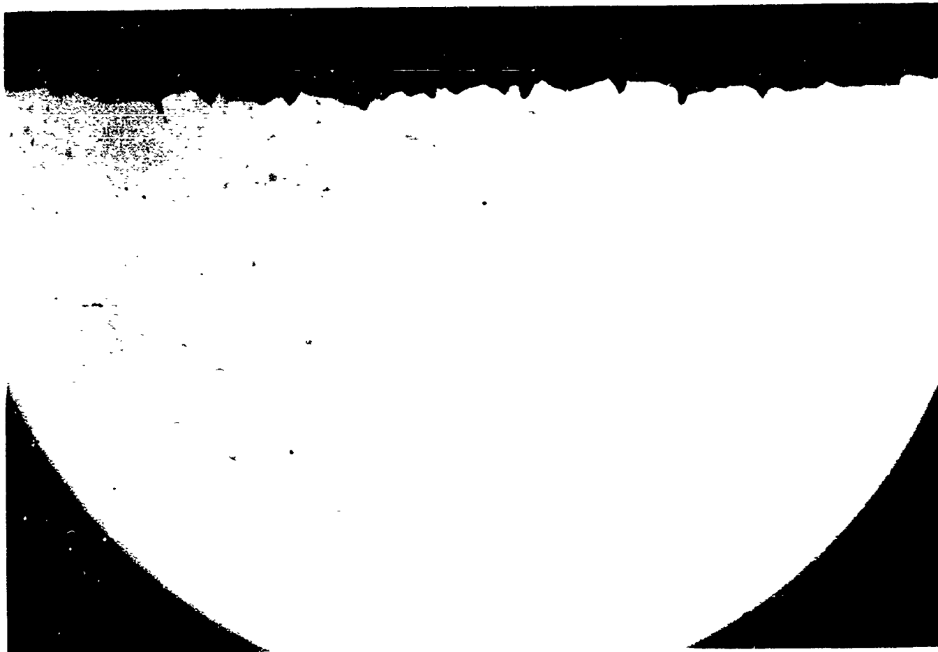
Fig. 26 Nickel-10% chromium alloy coated with sodium sulfate exposed to dry oxygen at 855°C for 16 hours (NC1-2a).
