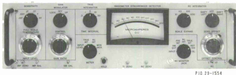
Fig. III-6. Radiometer system, synchronous detector panel.
