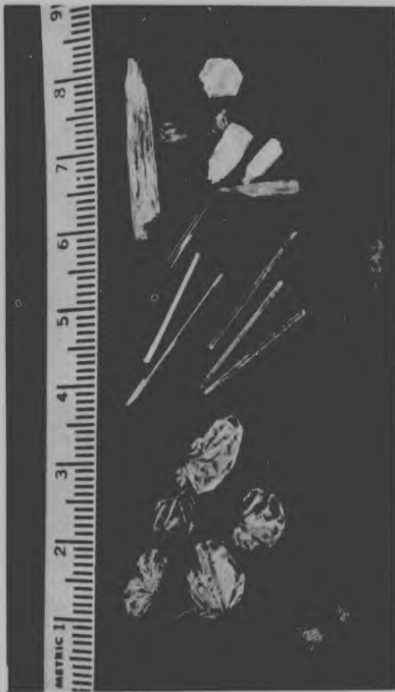
Fig. 3. Li- and Na-doped ZnO Single Crystals grown from ZnSe powder as a starting material.
