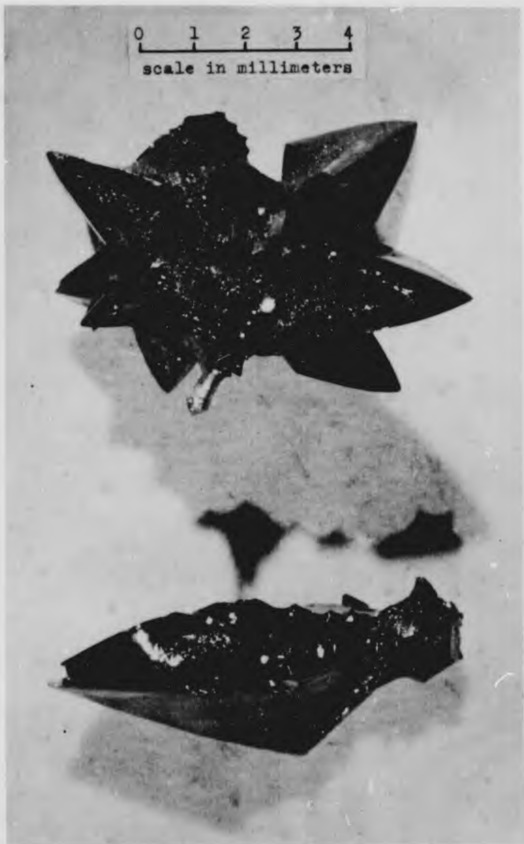
Figure 3. Single Crystals of Sm 0.99 WO 3
