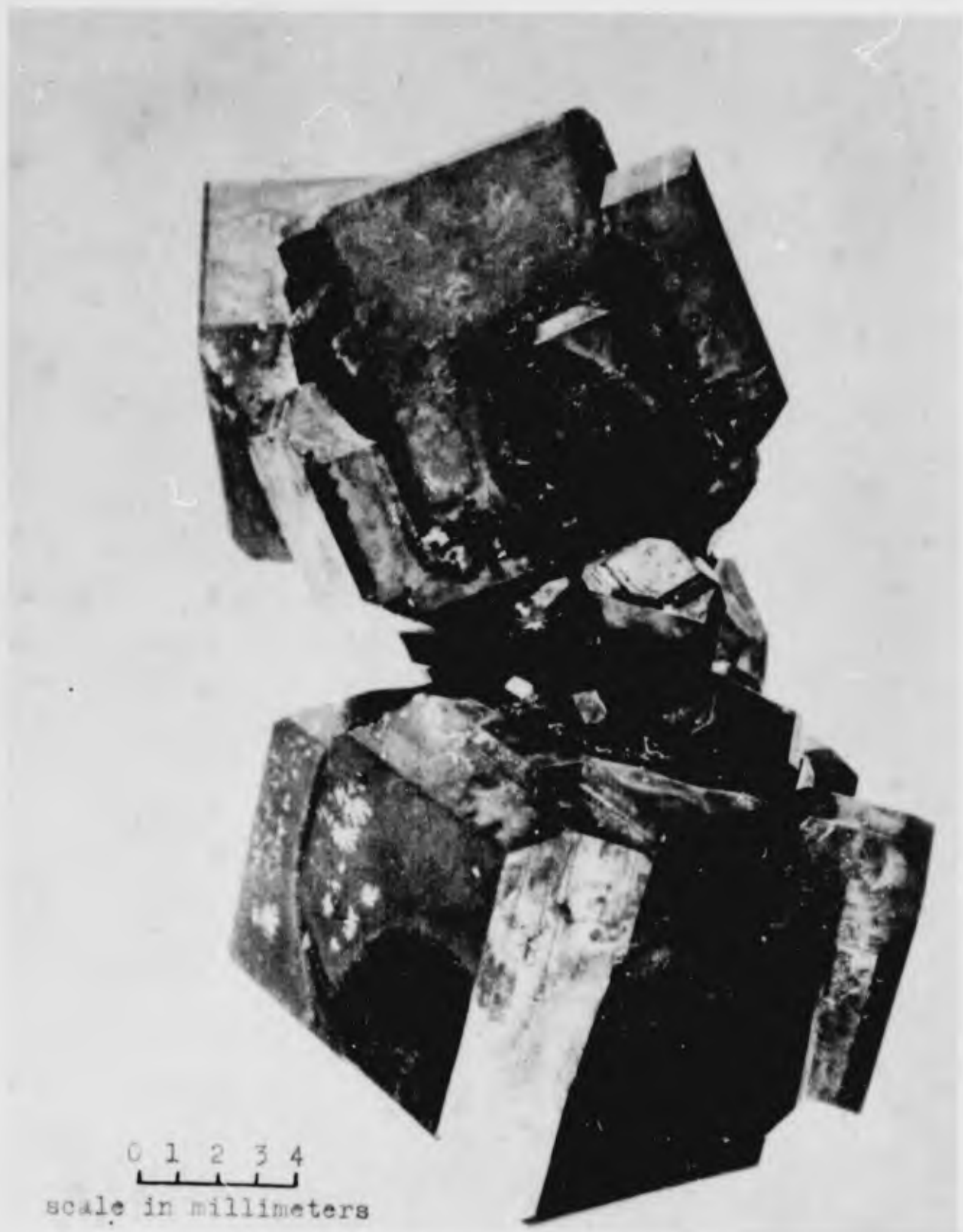
Figure 2. Single Crystals of \text{Na}_{0.65}\text{WO}_3
