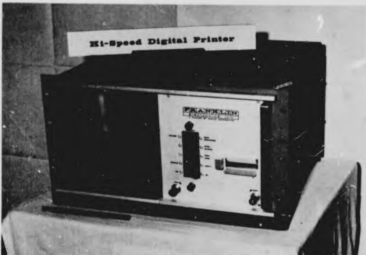
FIGURE 5 HIGH SPEED DIGITAL PRINTER MANUFACTURED BY FRANKLIN ELECTRONICS CORPORATION. THE UNIT IS CAPABLE OF PRINTING OUT 12 DIGITS EVERY 50 MILLISECONDS (240 CHARACTERS PER SECOND).
