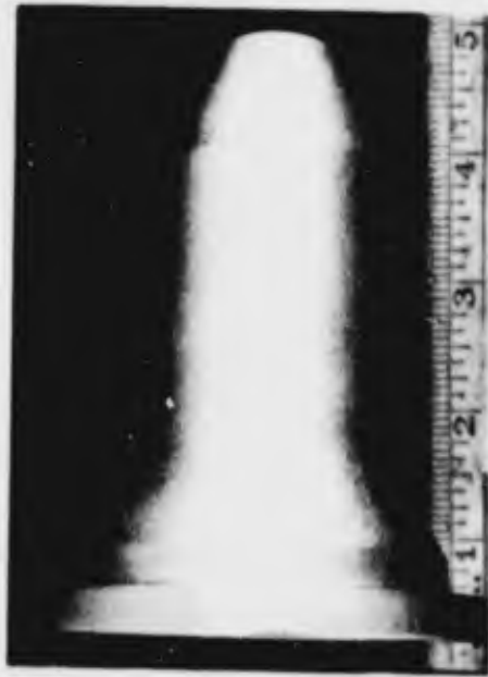
a. Small Nozzle Slurry-Coated with Hafnium-Tantalum Alloy (Sylvania Sylcor Div.)
