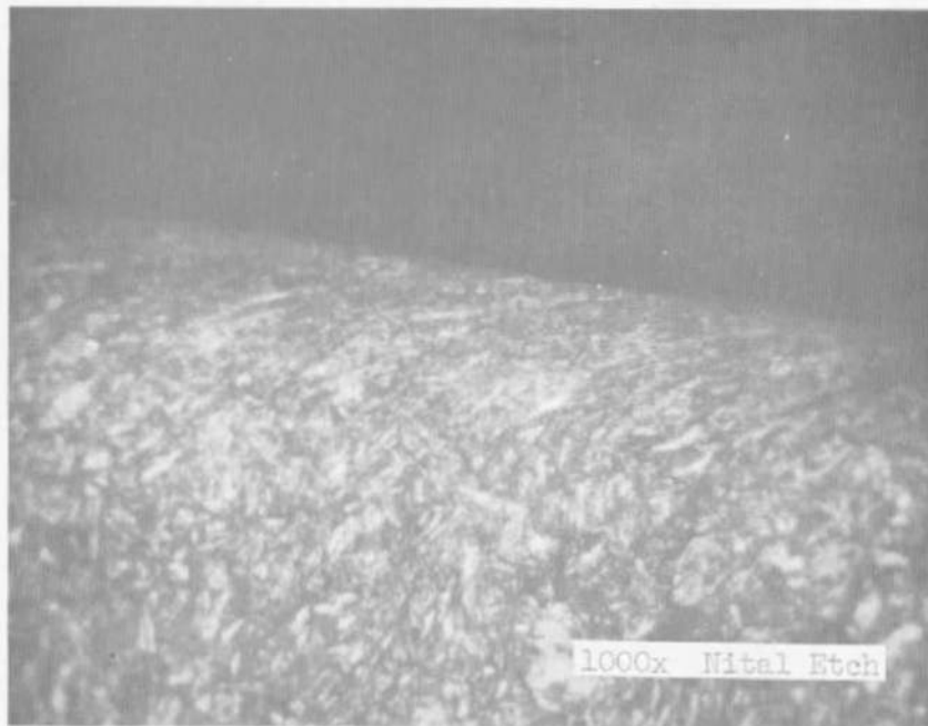
Fig. 5 Gun-Drilled Specimen after Tempering at 1000°F for 1/2 hr
