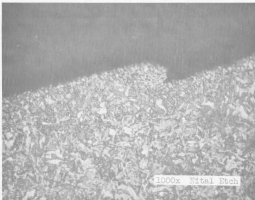
Fig. 6 Austenitized at 1425 for 20 min and Quenched in Water after Lathe Boring
