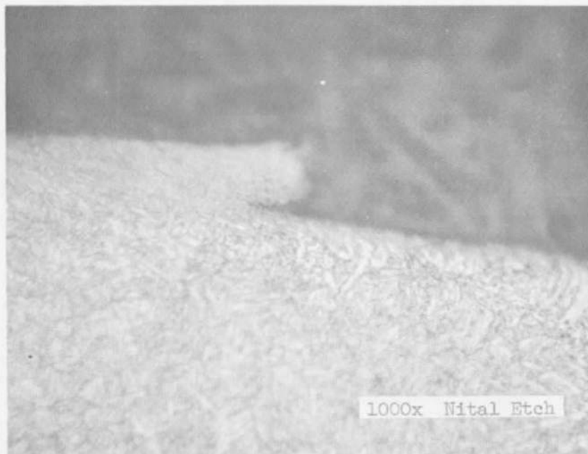
Fig. 2 Lathe Bored Using a Rex 95 High Speed Steel Cutter (Disturbed Layer Appears the Same as in Fig. 1)
