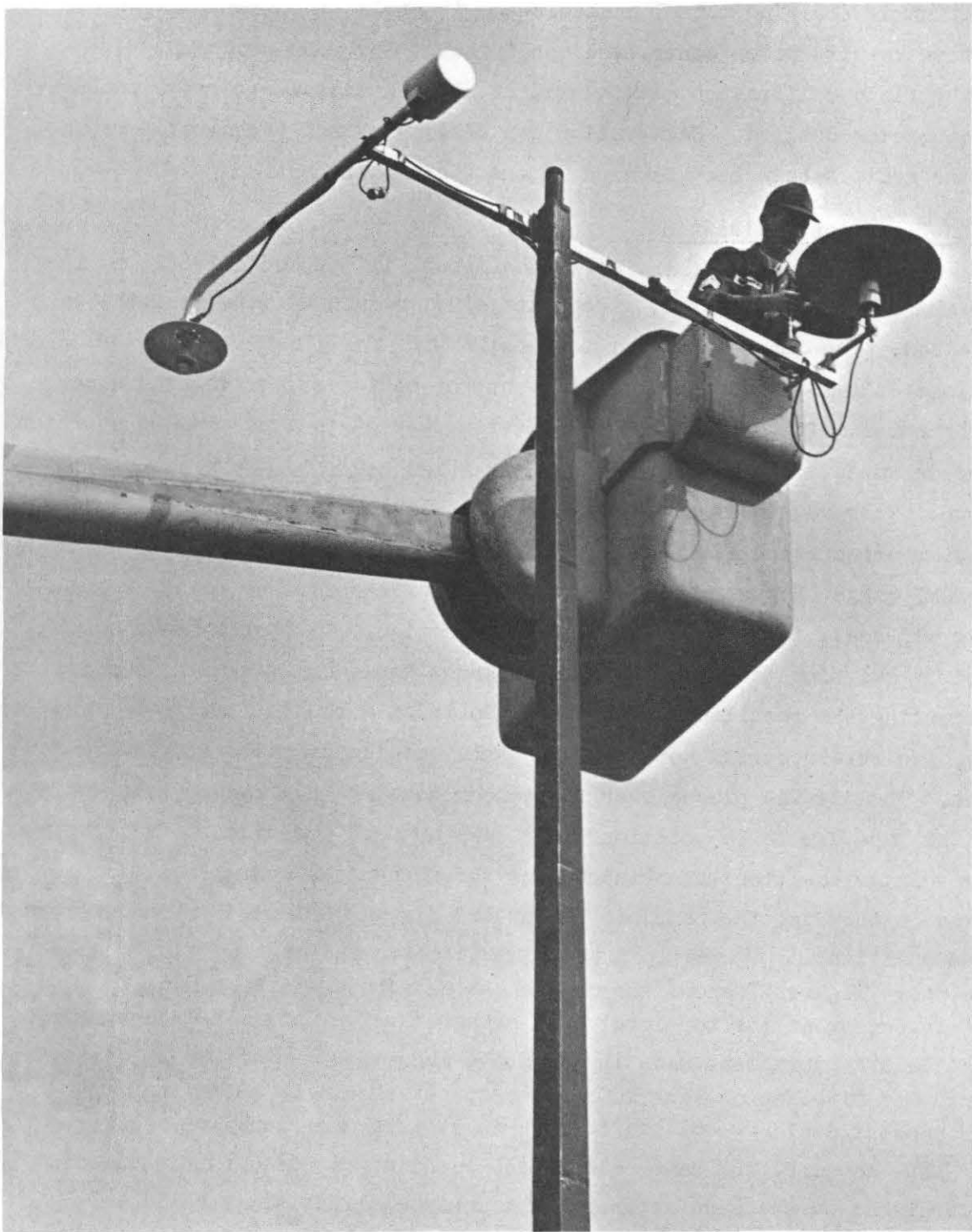
FIG. 17 - ON-SITE CALIBRATION OF WIND DIRECTION SENSOR USING JIG
