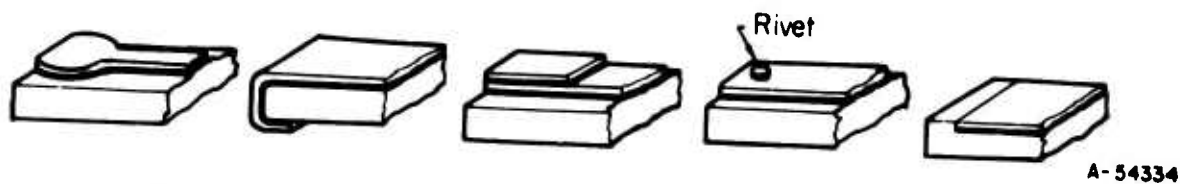
FIGURE 10. PEEL-RESISTANT DESIGNS FOR FLEXIBLE MEMBERS (Ref. 31)
