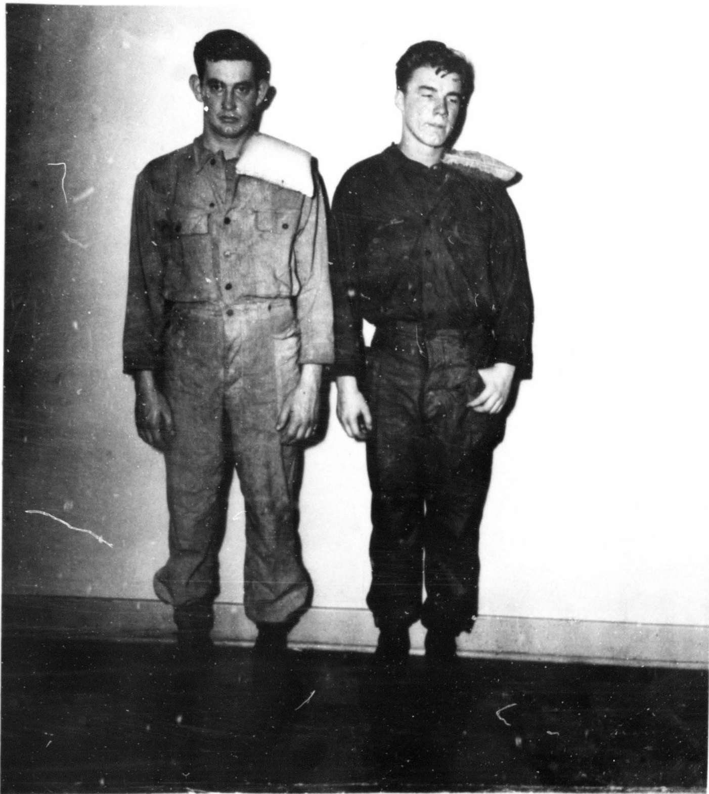
FP (D) FP (X) Appearance of flameproofed clothing (X) after ten wearings and flameproofed twill (D) after second wearing. ARMORED MEDICAL RESEARCH LABORATORY FORT KNOX, KY. Project No. T-5 Photograph #1
