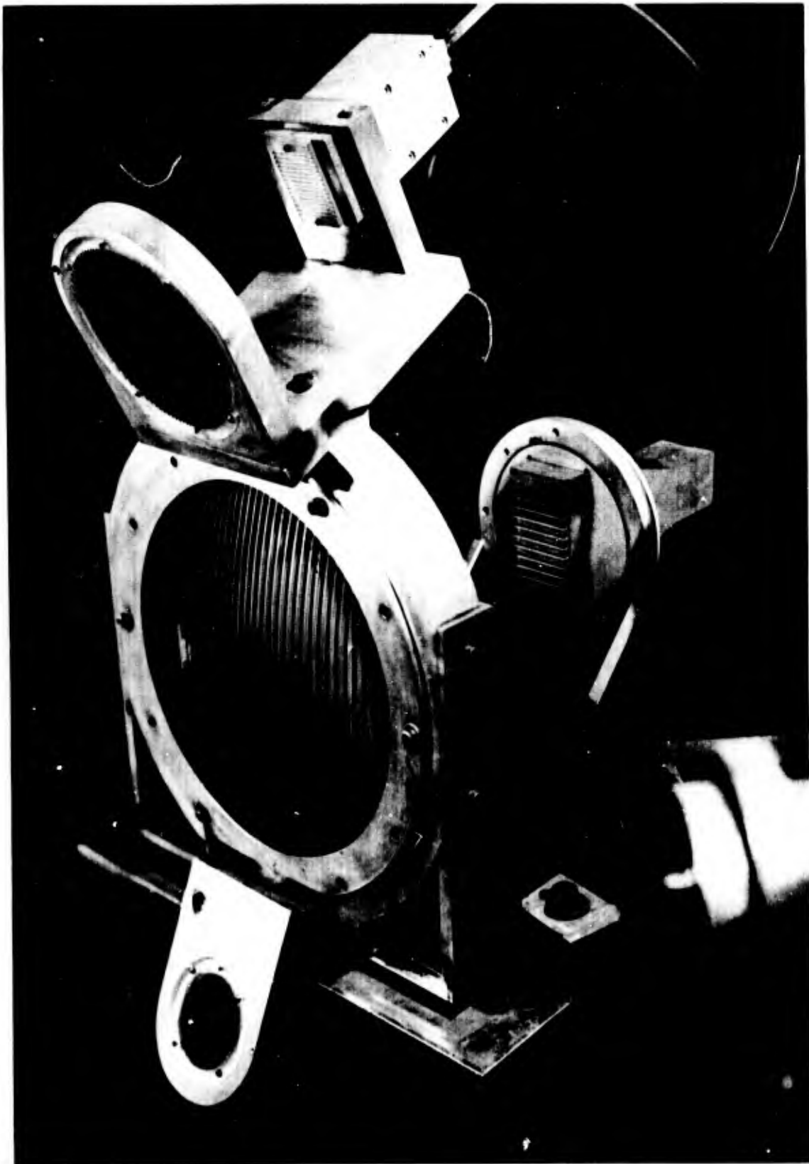
Fig.4 Antenna for 17GHz, 35GHz, and 70GHz Radars
