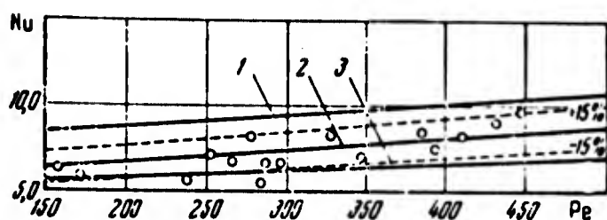
Fig. 4. Change of Nu from Pe during motion of liquid Al in graphite pipe d = 7.2 mm. 1 - Nu = 7 + 0.025 Pe^{0.8} ; 2 - Nu = 5 + 0.025 Pe^{0.8} ; 3 - Nu = 4.8 + 0.014 Pe^{0.8} ; 4 - Experimental points (Al).
