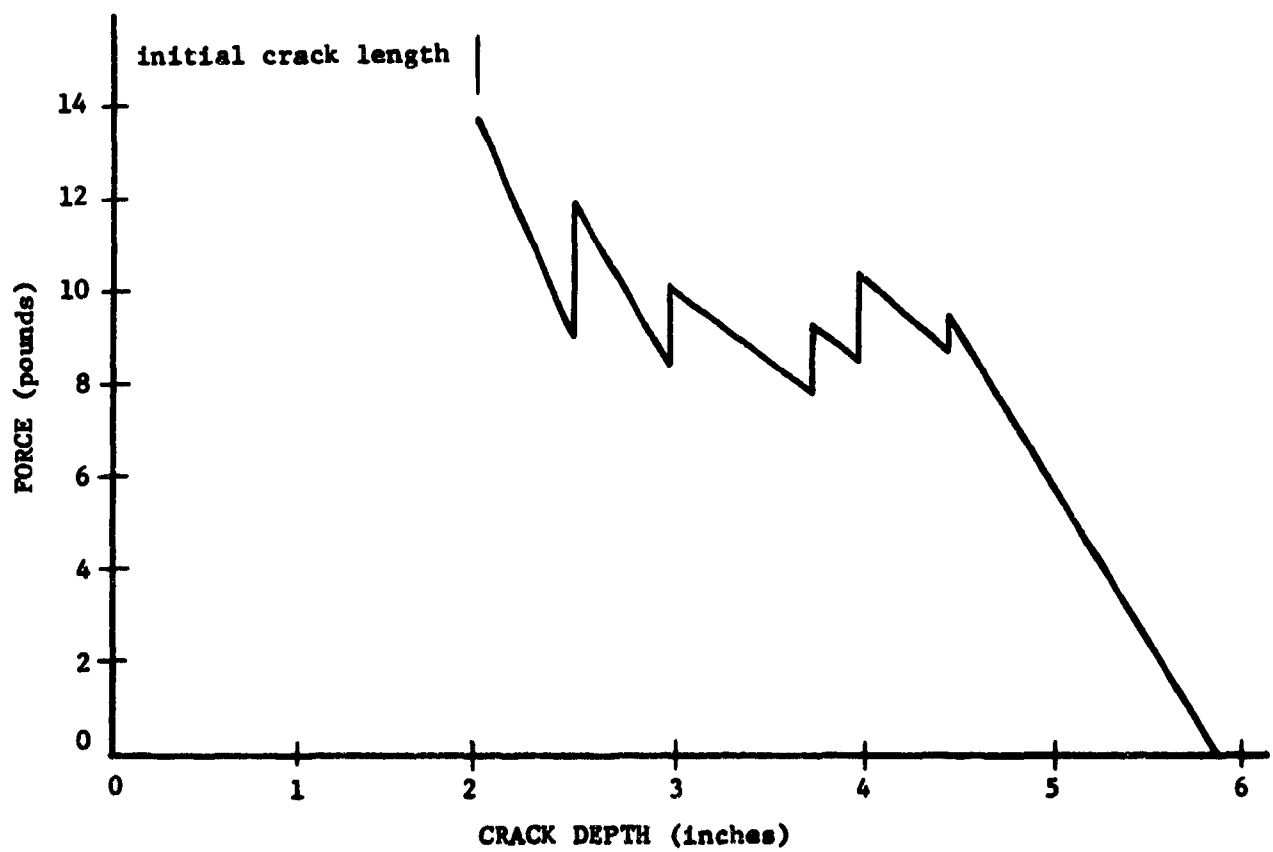
Fig. 10. Typical relationship between force and crack depth in double-cantilever specimen without embedded fibers.
