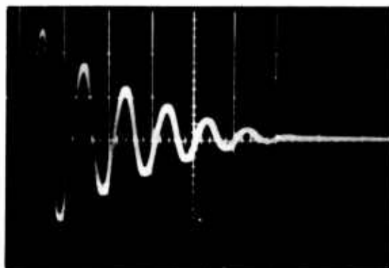
Figure 13. Typical current oscillogram. Scale 20 kiloamperes and 5 microseconds per large division.
