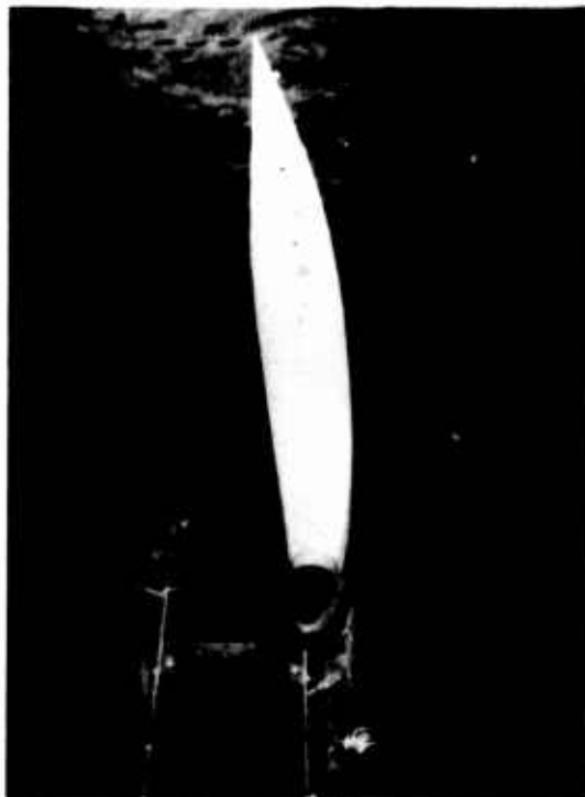
Figure 22. A deflector was added to the wind tunnel plexiglass chute to change the direction of air flow over the vent scoop and thus vary the effective angle-of-attack.
