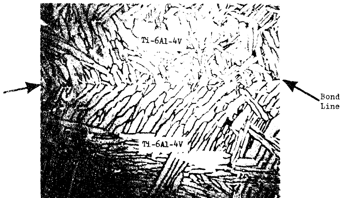
Figure 18. Run 3HP. Bonding at 1540°F; 650 psi; 1 Hour. Shear Strength: 81,470 psi. Met.-7444-2-2. Etched. 500X.
