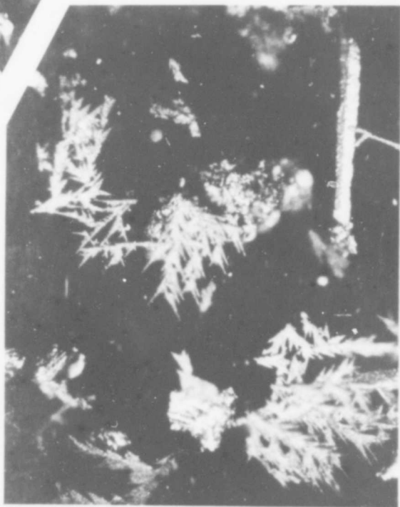
Fig. 9 Hafnium carbide needle dendrites and crystal from Run L. 450X
