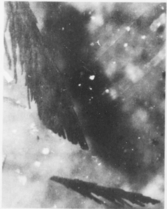
Fig. 14 Branched spikes after etching in \text{Hf-HNO}_3 . 29X
