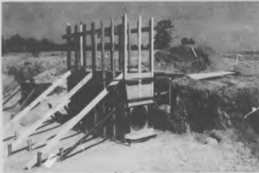
Fig. 13. Sandbox prepared for test loading; height of walls about 6 feet.
