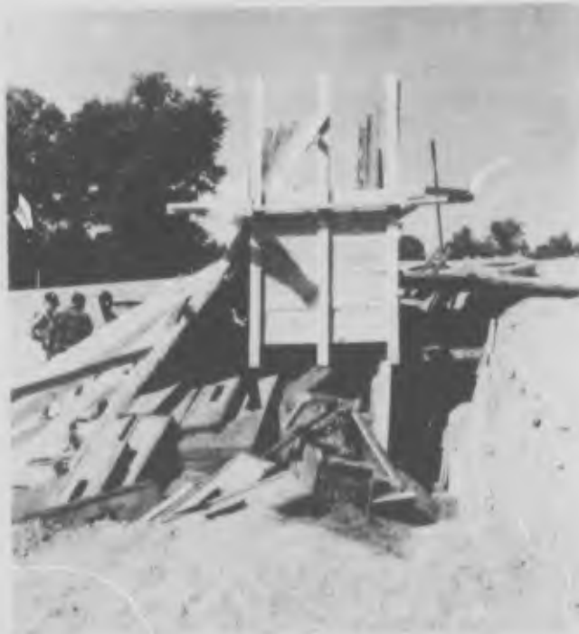
Fig. 32. Test installation viewed from south end after collapse of wall panel; Ring No. 1 buried under debris.
