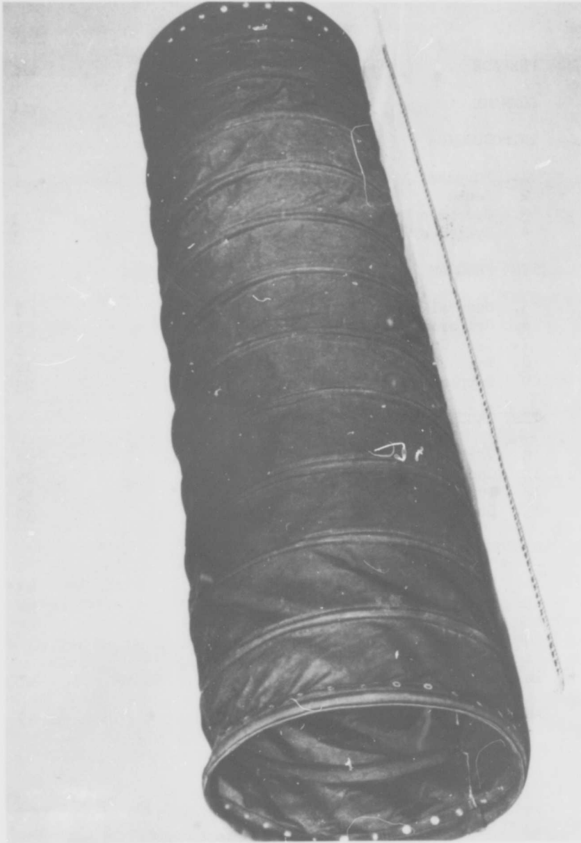
Collapsible canvas liner for shallow tunnels.
