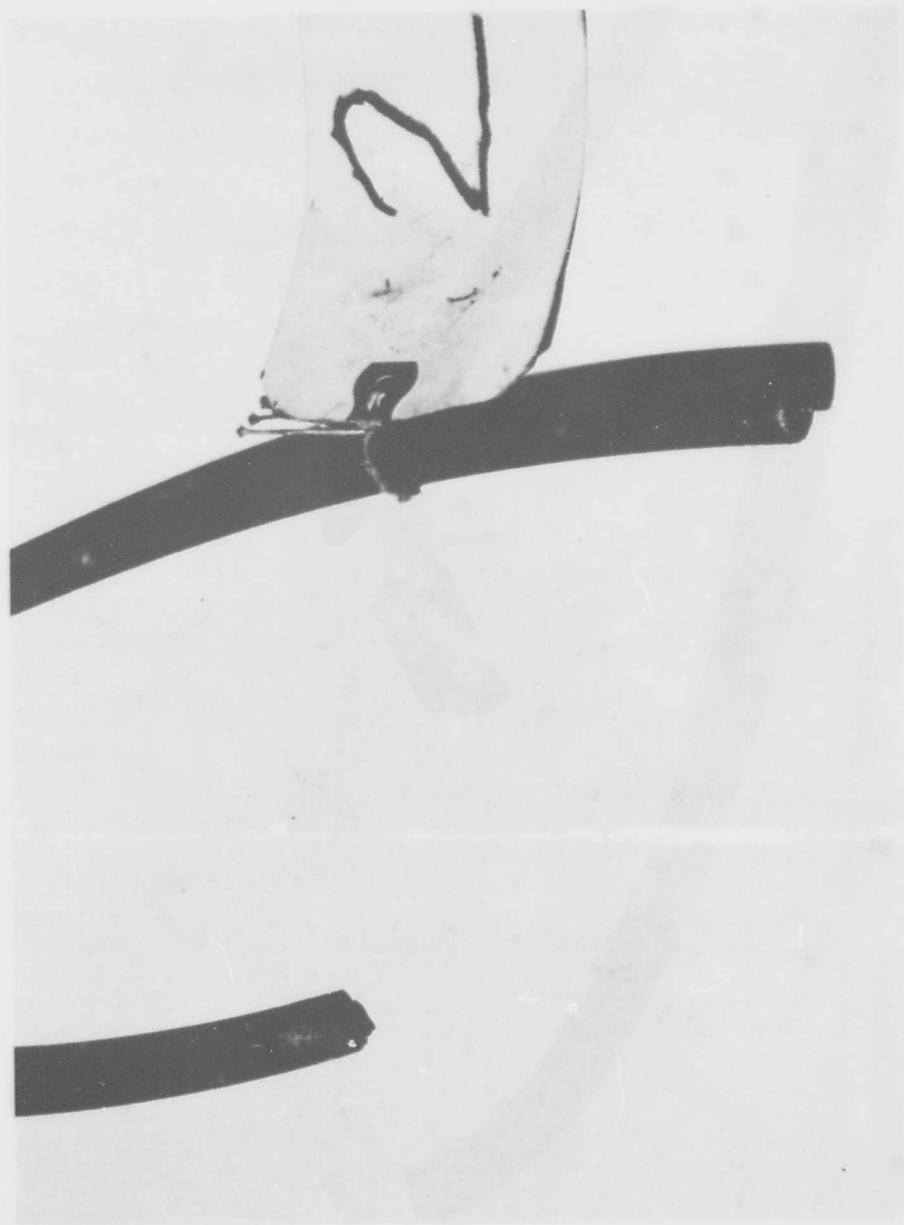
Fig. 37. Ring No. 2 joint failure caused by excess bending stress in pipe insert.
