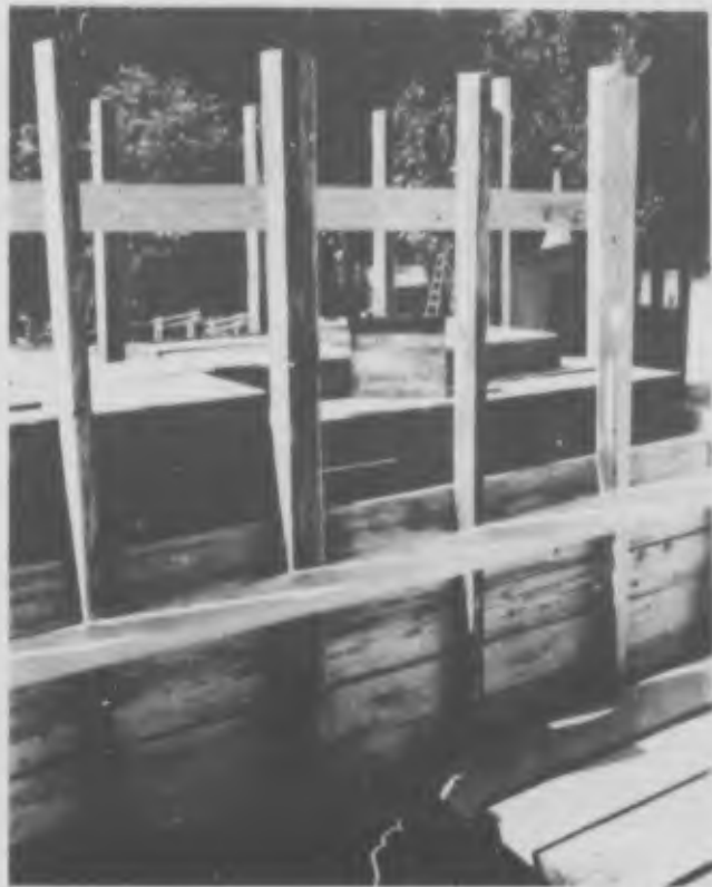
Fig. 21. Test load at 8-ton surcharge level.
