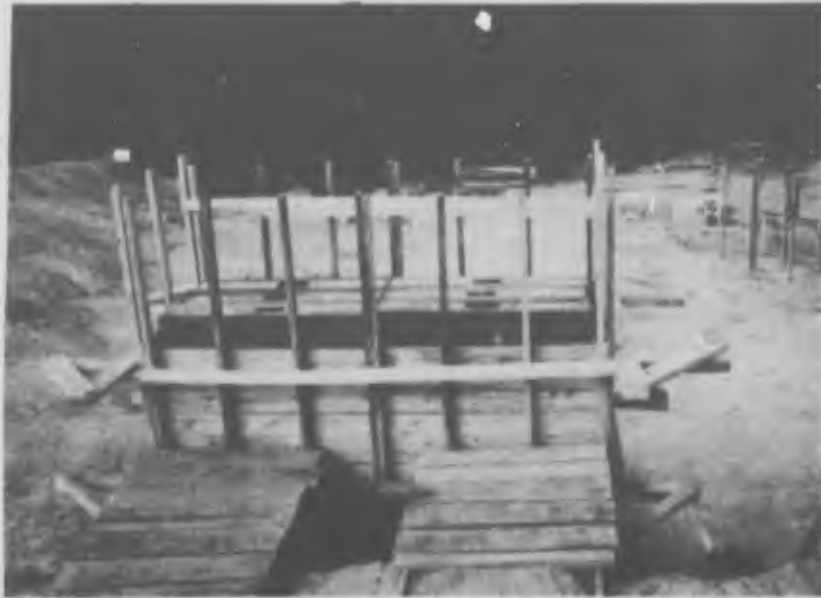
Fig. 19. Six-ton surcharge covering complete surface of sand fill (note levelness of weights).
