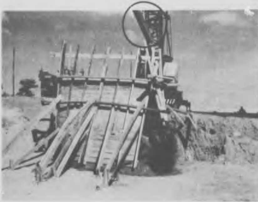
Fig. 29. Failure of sandbox at 13\frac{1}{2} -ton surcharge level (note additional 1,000 pounds being applied). F8069
