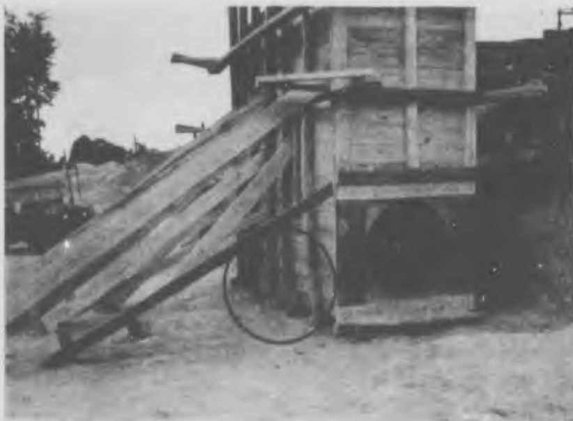
Fig. 28. South end of sandbox at 12-ton surcharge level (note splitting of wall studs and addition of jury braces).
