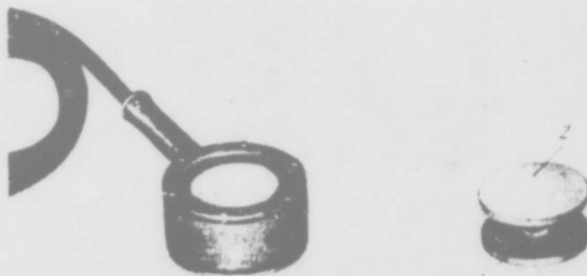
Fig. 83. Sound receiver and piezoelement with receiving ceramic diaphragms. 1) housing of the sound receiver; 2) diaphragm; 3) cylindrical piezoelement.
