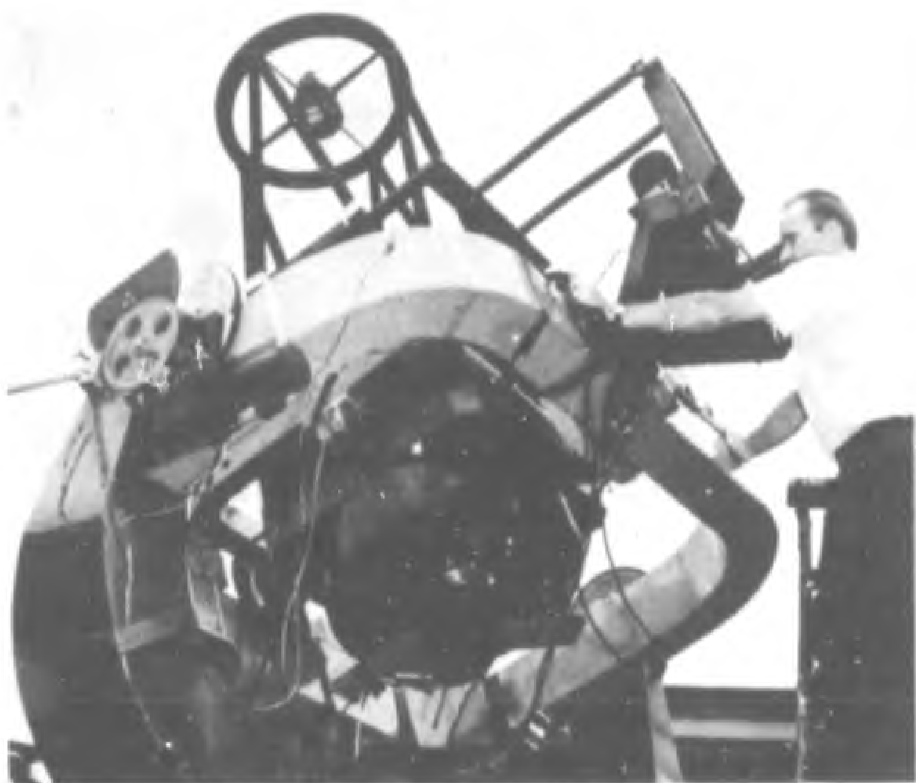
Figure 2. ARL 4-axis, 24-inch satellite tracking telescope.
