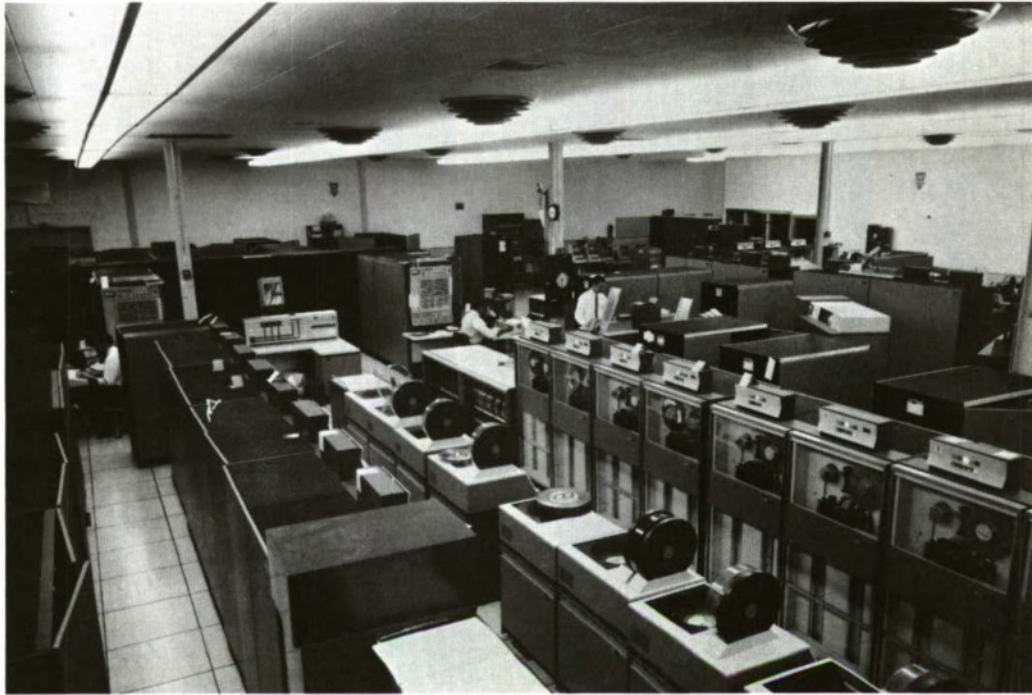
Lincoln Laboratory Computation Center, showing IBM 360/67 computer with two central processing units (upper left) and three core memory modules, and (upper right) a 360/40 used in support of the 360/67. A number of individual time-sharing consoles are in regular use at remote locations in the Laboratory.
