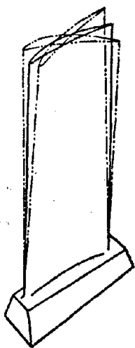
Fig. 5.2. One-node form of torsional vibrations of a blade.
