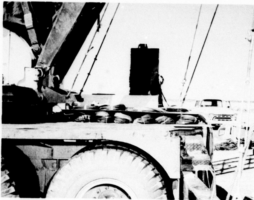
Figure 17. Umbilical Cable Pay-Off System
