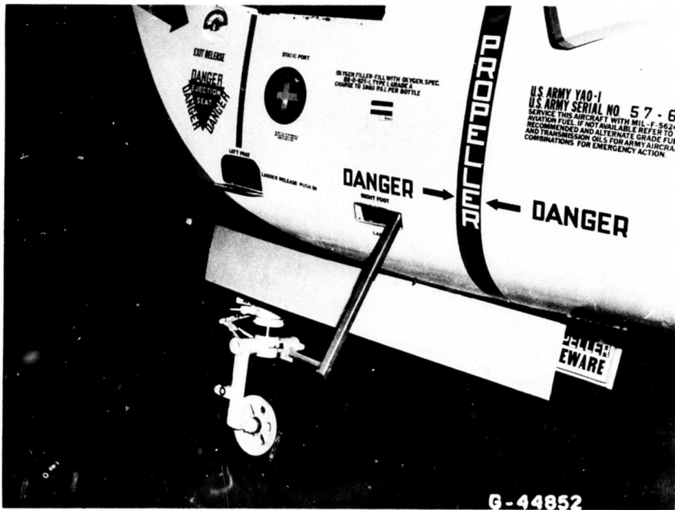
Figure 6. View of the exterior rescue and danger area markings.
