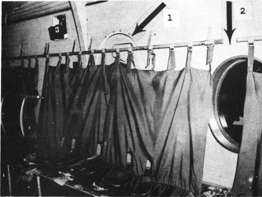
Figure 21. The present emergency exit location in the cabin (arrow 1) necessitates removal of the upper seat structure before it can be used. Location of the exit between two adjoining seats (arrow 2) would simplify evacuation.
