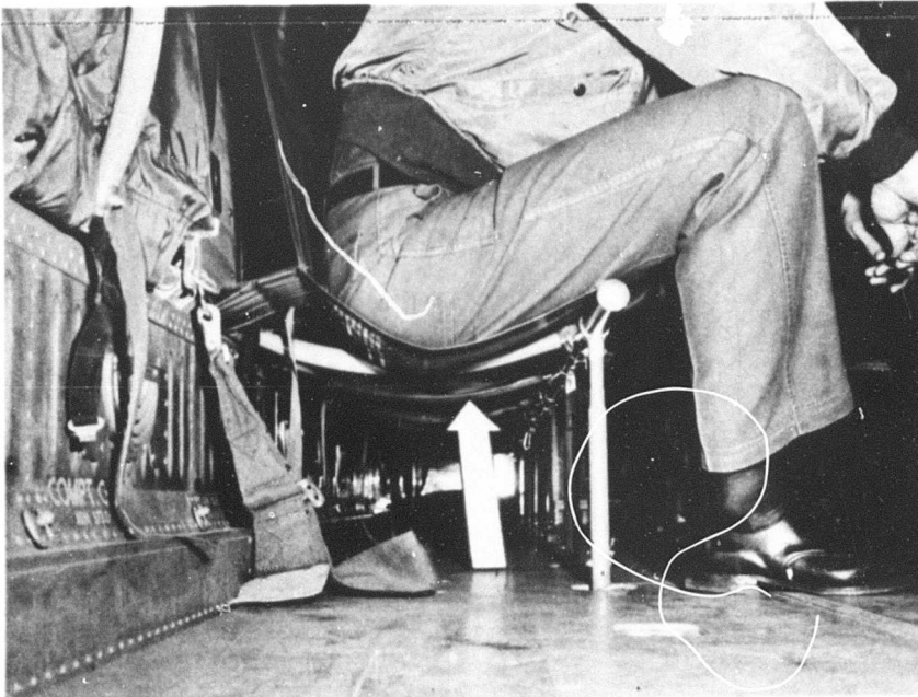
Figure 13. Close-up showing the load distribution over the front and rear support tubes and seat back. The arrow indicates where the occupant straddles the spreader.
