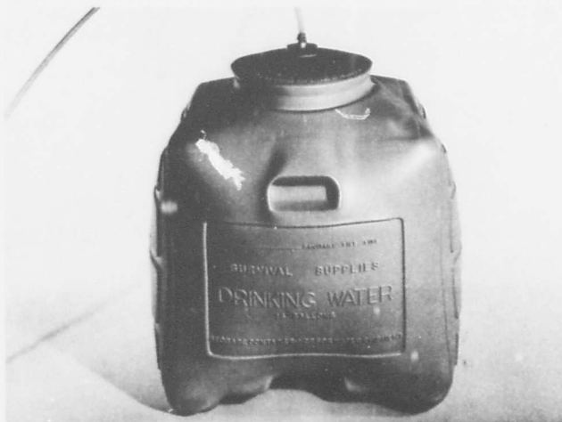
Figure 23 CONTAINER WITHOUT FRAME AT 30 PSI PRESSURE
