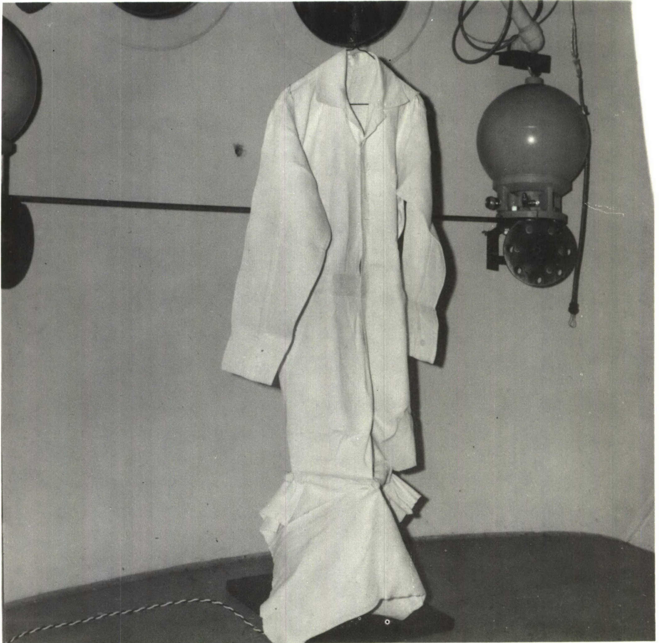
Fig. 7 Typical Pre-Fire Conditions , Hyperbaric Chamber
