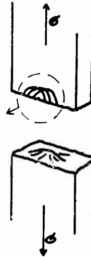
FIG.7.21 SYMMETRICAL SHEAR BAND PATTERN NEAR A FRACTURE SURFACE SUPERPOSED ON THE PATTERN OF BANDS MORE COMMONLY OBSERVED(PMMA, LOT 1)
