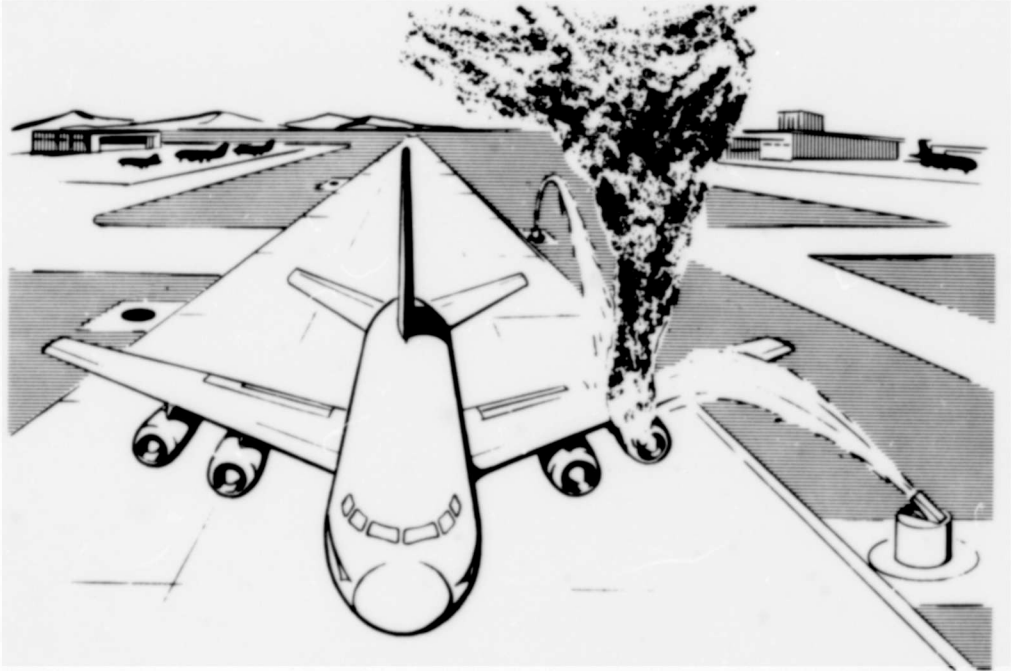
Figure 8. Remote Controlled Pop-up Nozzle Fire Suppression System at Airport
