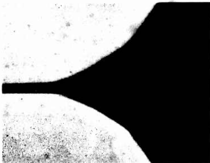
Figure 1a. Enlargement of expansion region of Figure 1. Note that the vapor veil is penetrated by the backlighting. Luminosity from the interior is seen just after voltage peak
