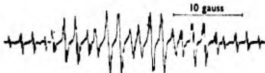
E.s.r. spectrum of radical (I) from the photolysis of 1 \times 10^{-3}M -phenalen-1-one in propan-2-ol.
