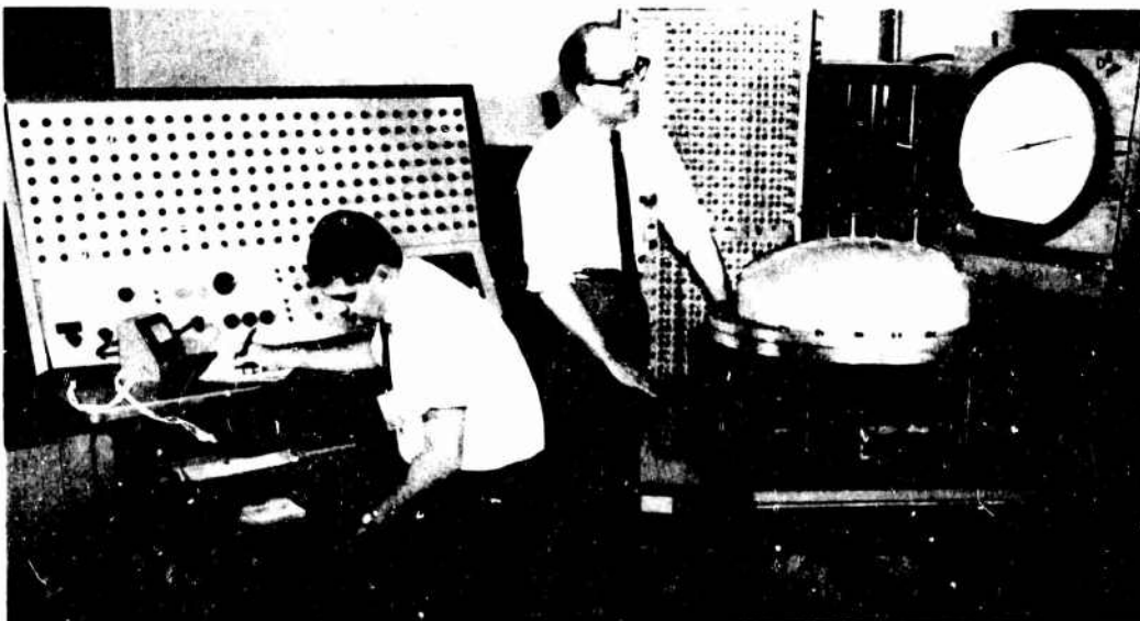
Figure 7. TEST SETUP FOR STRAIN MEASUREMENTS ON TORISPHERICAL SHELLS UNDER INTERNAL PRESSURE LOADING
