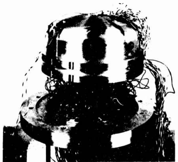
Figure 12. MACHINED 7075-T6 AL TORISPHERICAL SHELL MODEL - 9.68" BASE DIAMETER - WITH BASE FIXTURE
