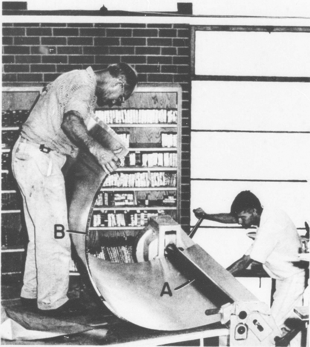
Figure 23. Rolling of Honeycomb Core: A, Center Roller; B, Edge of Core and Protective Sheets.
