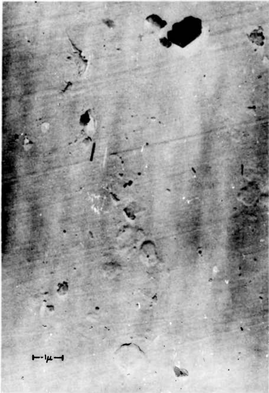
FIGURE III-2. Shadowed carbon replica of the surface of type No. 1025 Daicel plastic. The numerous surface inclusions and striations are characteristic of the commercial plastics.
