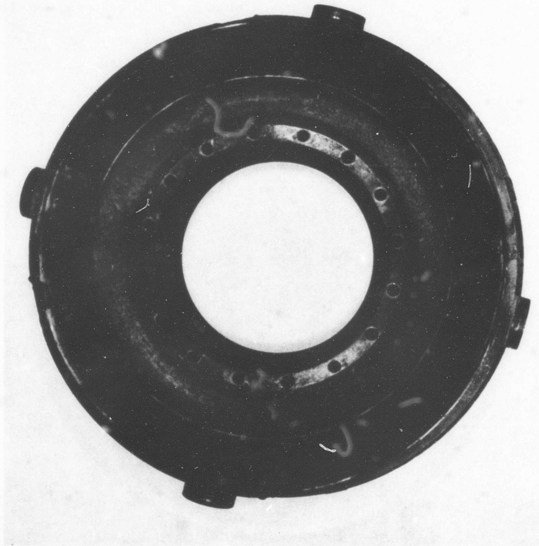
Figure 29. First-Stage Nozzle, Leading Edge, Post-Test Condition.
