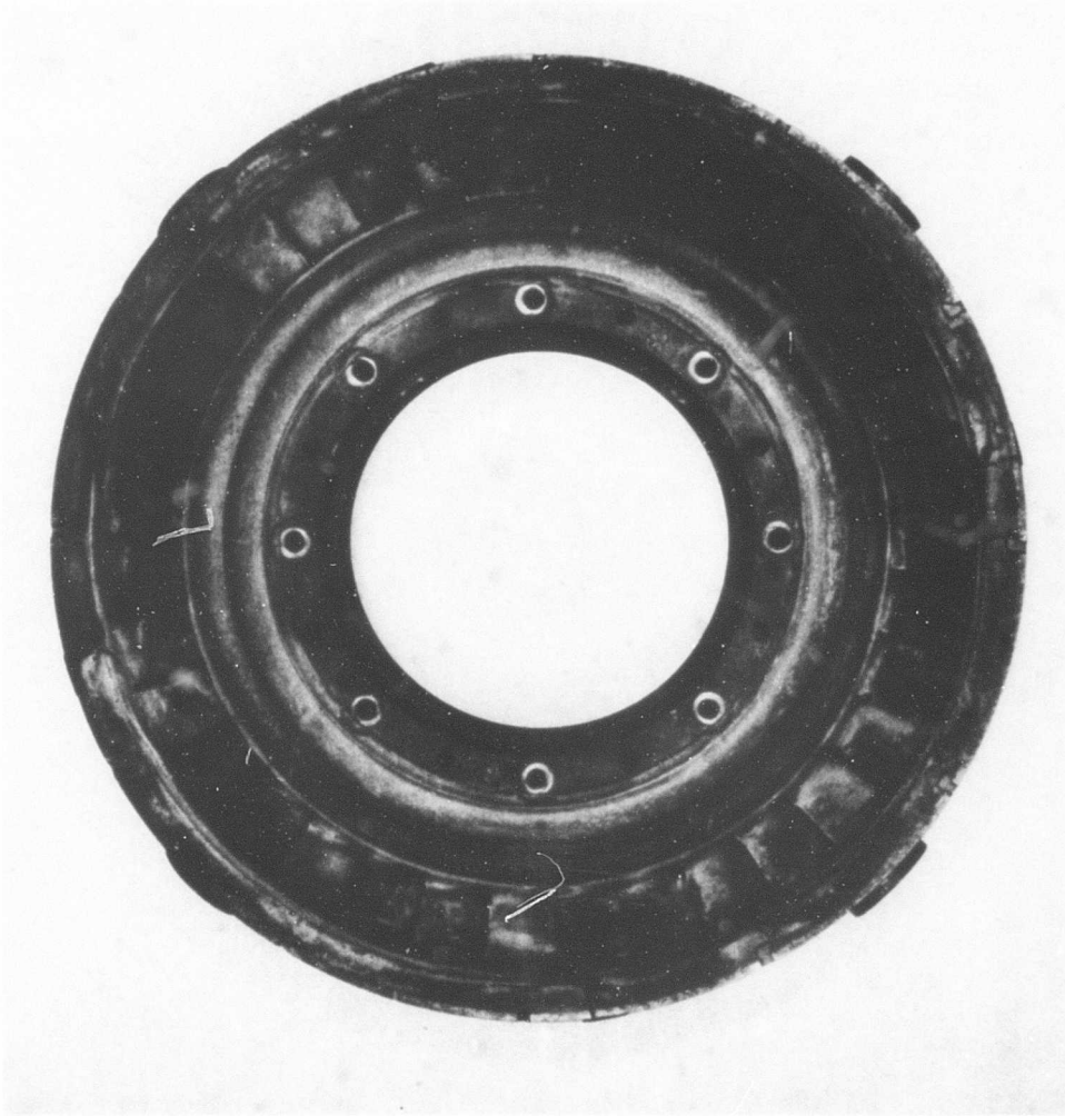
Figure 30. First-Stage Nozzle, Trailing Edge, Post-Test Condition.
