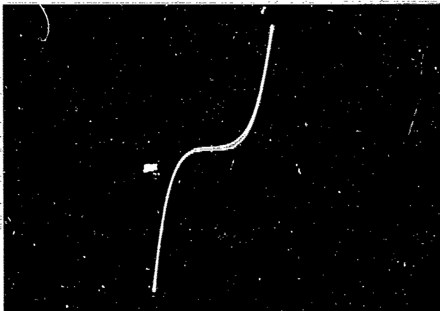
Figure 4. 60-Hertz I-V characteristic of five-layer Schottky diode. Horizontal scale, 5 v/cm; vertical scale, 1 ma/cm; T \sim 300^{\circ}\text{K} (sample 3).
