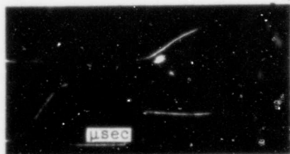
Fig. 2. Combined in time frame of glow, taken through a transverse slot 46 \times 0.5 mm 2 , and oscillogram of pressure, recorded by a piezotransducer embedded in lateral wall of tube strictly opposite slot. Narrow luminescent band on frame is obtained during passage of perturbation through auxiliary slot 4 \times 0.5 mm 2 , located 23 mm ahead of basic slot. A light signal, passing the auxiliary slot simultaneously is recorded by the PM.
