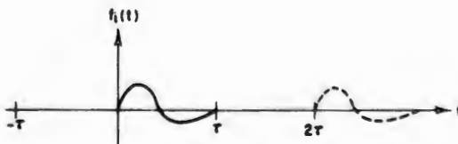
FIG. 6.7. A transient excitation artificially converted to a periodic excitation with period 2\tau .
