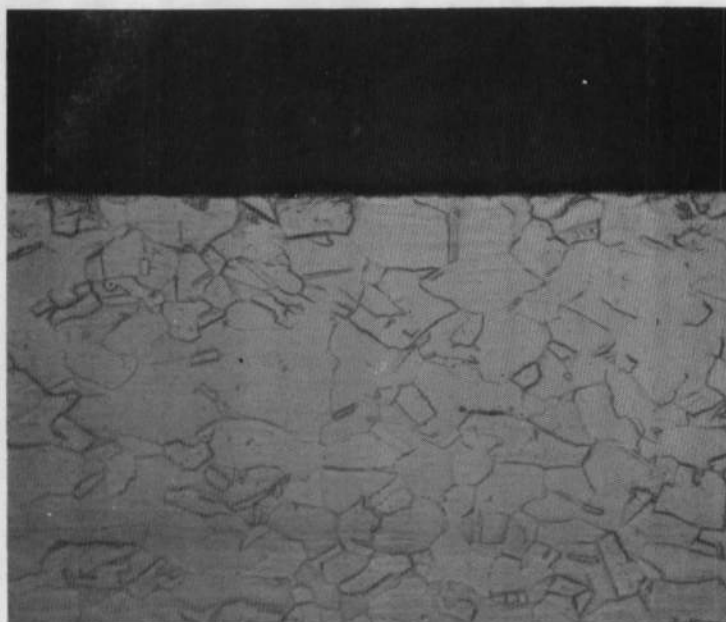
Fig. 25 Copper Shim Portion of Composite Specimen, Away from Weld, Exposed to F_2 , Stressed, 500X
