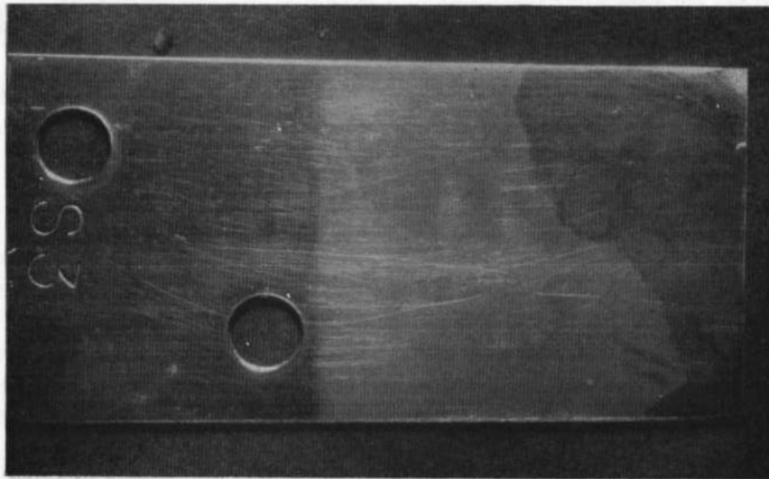
Fig. 6 Unwelded Stainless Steel 304L, Exposed to F_2 , 2X
