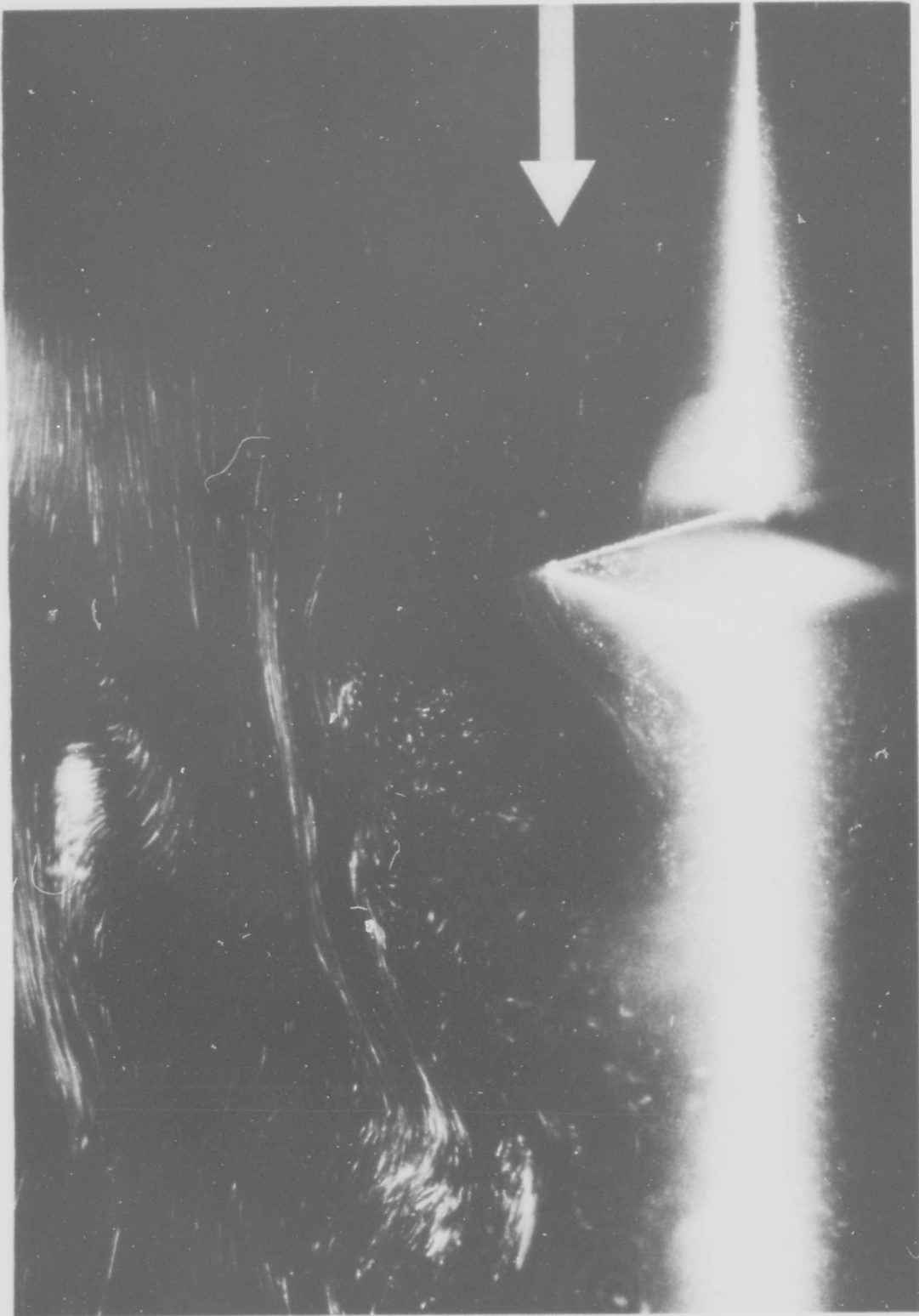
Fig. 5. Lee waves and rotors behind a ridge in a stably stratified flow ( Ri=13 , Re=914 ). Upstream velocity and density gradient are constant. (See Fig. 4 caption for other details).
