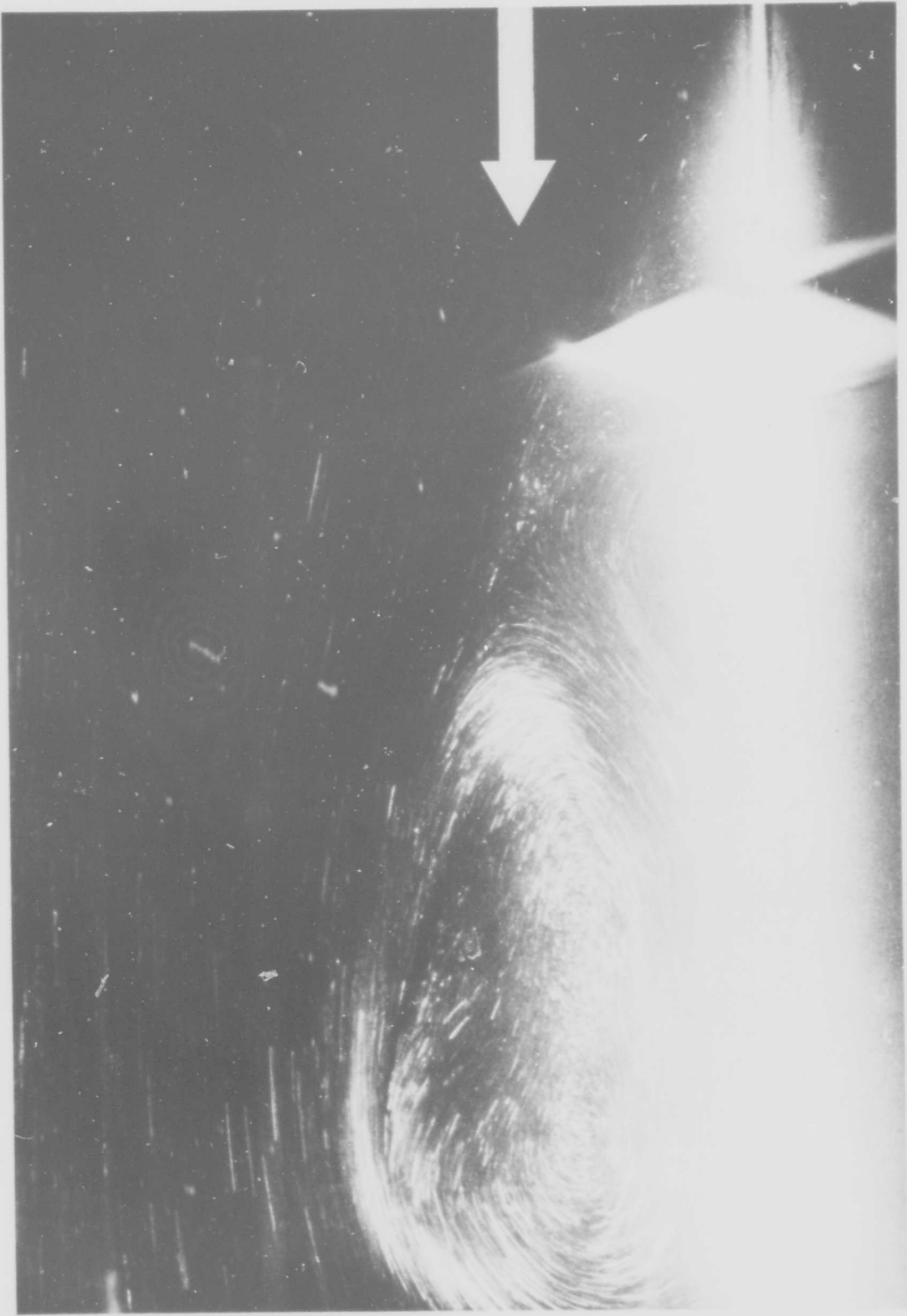
Fig. 6. The eddy behind a ridge in a homogeneous fluid ( Re=914 ). (See Fig. 4 caption for other details.)
