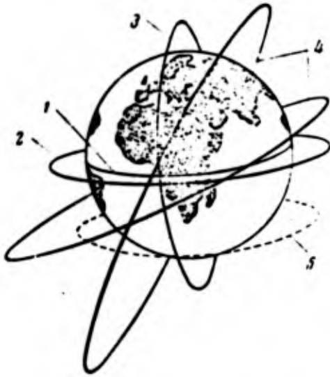
Fig. 57. Possible orbits of communication satellites. 1 - equator; 2 - equatorial orbit; 3 - polar orbit; 4 - intermediate orbits; 5 - unrealizable orbit.
