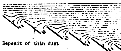
Fig. 10. Field of flow in a louvered dust separator.
