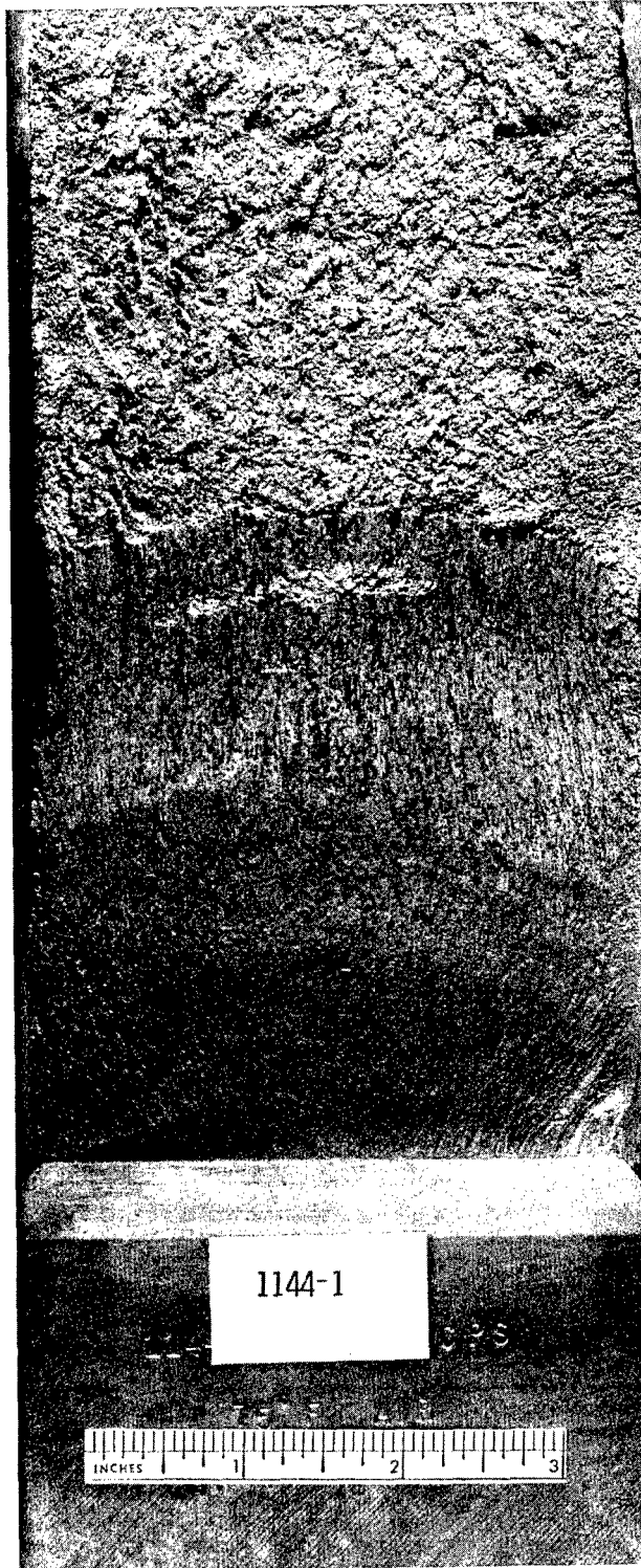
Sec. 7 Fig. 20—Room temperature fatigue fracture appearance of AISI 1144 steel (4T WOL Specimen)
