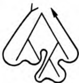
Fig.1—Tree walk using a push-down stack
