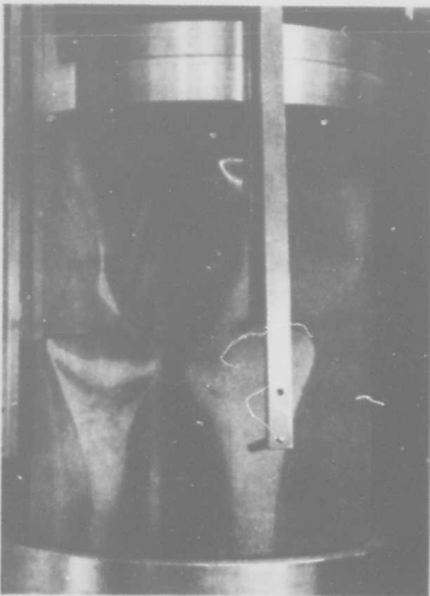
c. Collapse, Unpressurized
