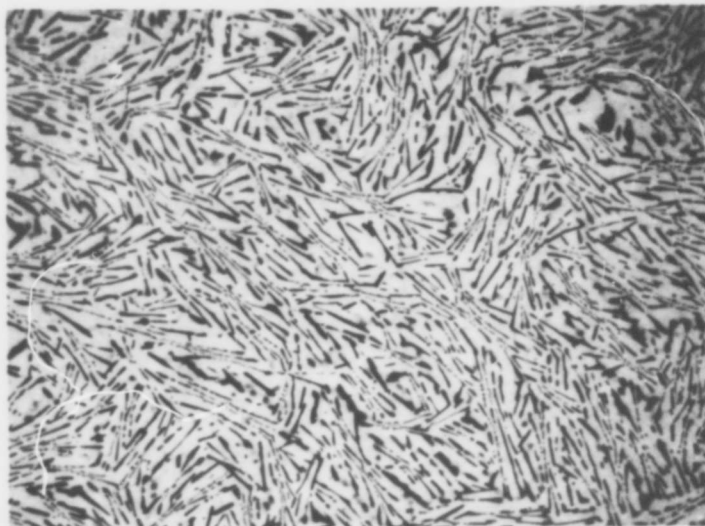
Figure 35. Nb-W-C (33-11-59 At.%), Melted and Rapidly Cooled X400 Monocarbide + Graphite Eutectic-Type Structure.
