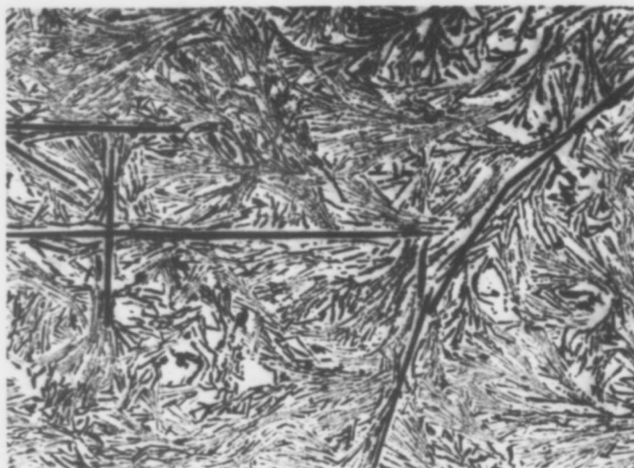
Figure 34. Nb-W-C (34-6-60 At.%), Rapidly Cooled From \sim 3300^{\circ}\text{C} . X130 Small Amounts of Primary Graphite in Monocarbide + Graphite Eutectic Matrix.
