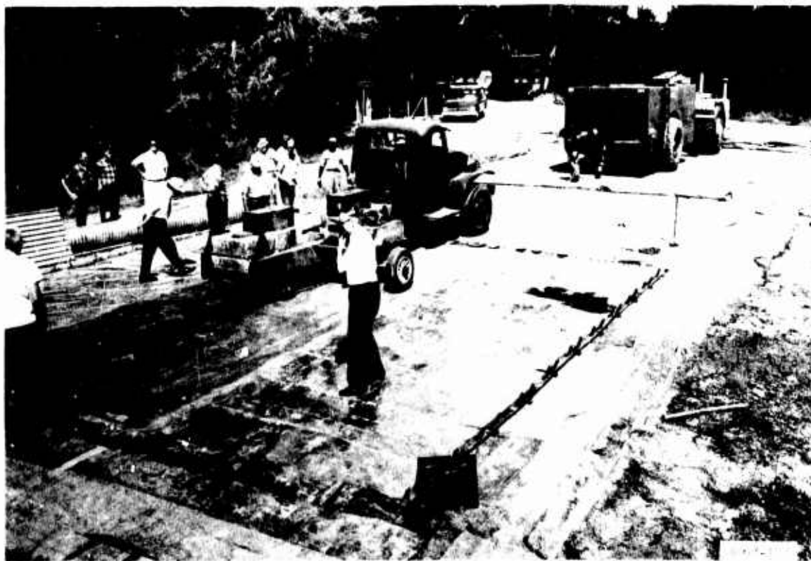
Photograph 16. Test 3; skid test in progress on steel membrane
