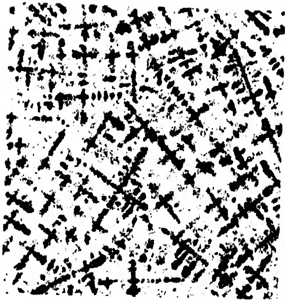
A) Sectioned perpendicular to primary axes of dendrites. No homogenization. Primary arm spacing 254 \mu .
