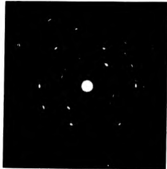
A) Tempered Martensite - Unaffected Area
