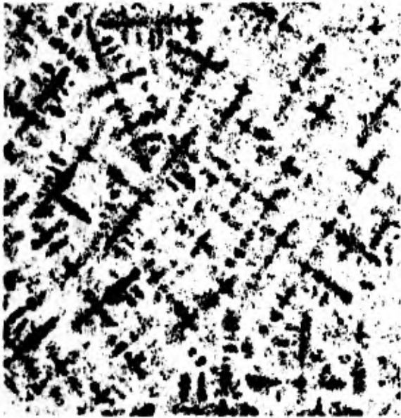
A) Sectioned perpendicular to primary axes of dendrites. No homogenization. Primary arm spacing 305 \mu .
